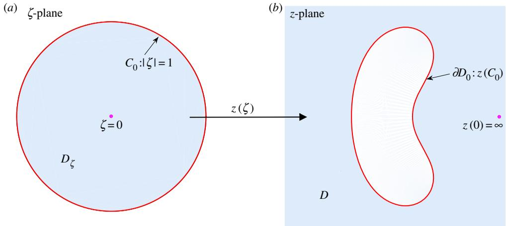
**Figure 1.** Schematic of the pre-image parametric  $\zeta$ -plane being the interior of the unit circle  $C_0$  (a), and the target image domain in the  $z$ -plane exterior to the bubble (b).
